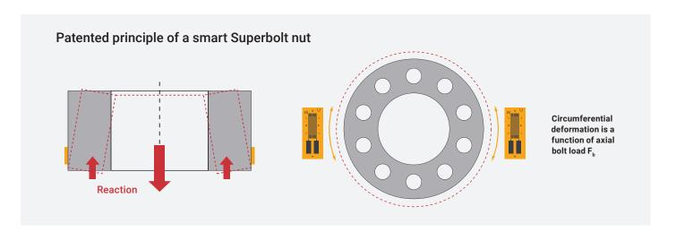
The principle of a preload monitoring Superbolt MJT or Flexnut relies on the ability to measure accurately the circumferential expansion of the nut body and to link it back to the preload level  $F_{\rm h}$  in the main bolt.
