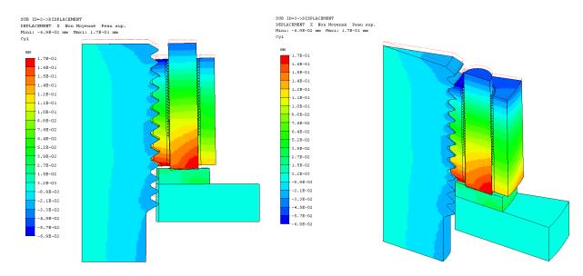
Deflection as shown by finite element simulation to choose optimal location for strain gauges
