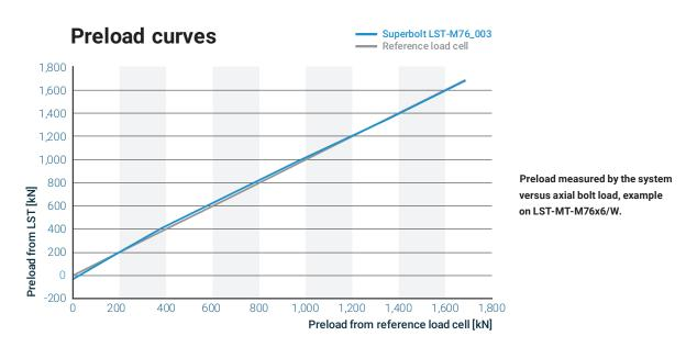
The value given by the smart Superbolt nut matched the preload measured by the calibrated load cell (reference cell). This performance matches the best accurate preload (± 2%) monitoring systems available commercially.
