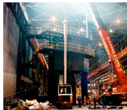
The world's largest bolt-style Superbolt being installed in a two-post hydraulic forging press.
